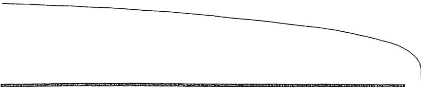
**Fig. 8.8.** Film flow over a horizontal plate.
