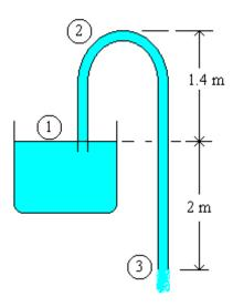
$$\frac{p_1}{\rho g} + \frac{v_1^2}{2g} + z_1 = \frac{p_3}{\rho g} + \frac{v_3^2}{2g} + z_3$$
