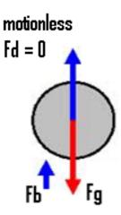
Since the system is stable and motionless, Newton's second law of motion reduces to:
