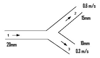
Total mass flow into the junction = Total mass flow out of the junction
