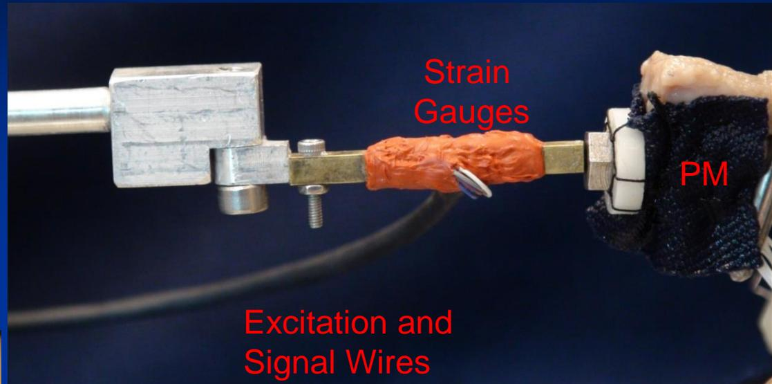
*(Top) Papillary muscle force transducers measure axial, and two directions of bending force on each papillary muscle*
