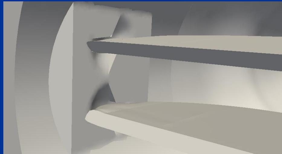
Interior view showing fully open leaflets fitting into butterfly hinge geometries
