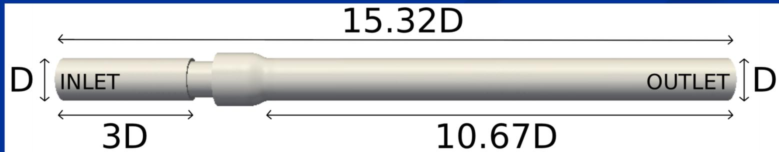
Computational model of experimental *in vitro* flow loop setup
