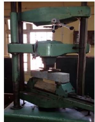
Fig 7: Flexural strength test
