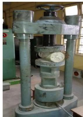
Fig 6: Split tensile strength test
