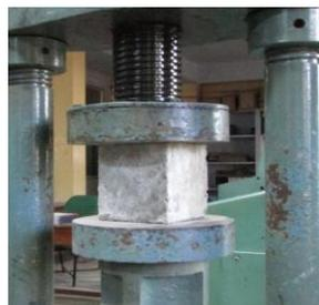
Fig 5: Compressive strength test
