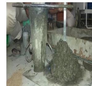
Fig 4: Slump test
