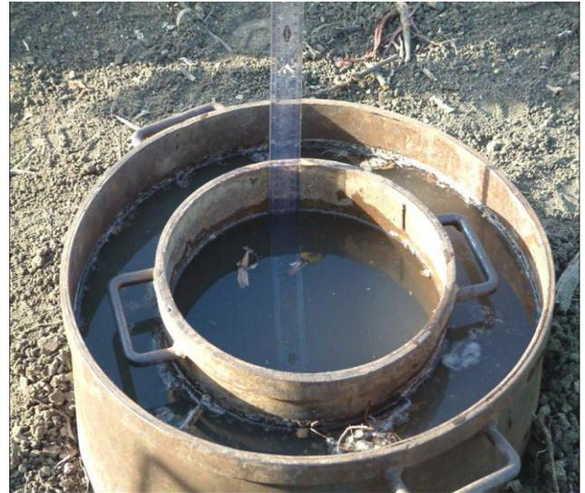
**Figure.2. Simple Double Ring Infiltrometer**
