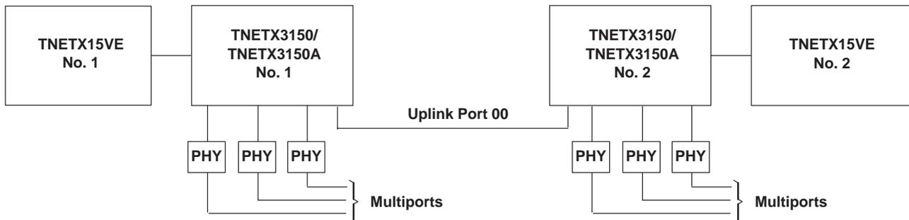
Figure 30. Cascaded Switches Through Uplink With Pretag Support
