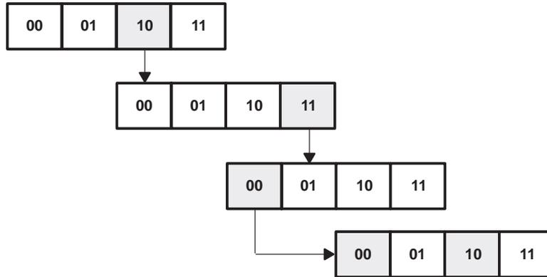
Figure 7. Example of Lookup-Number Algorithm (Adding 0xB0)
