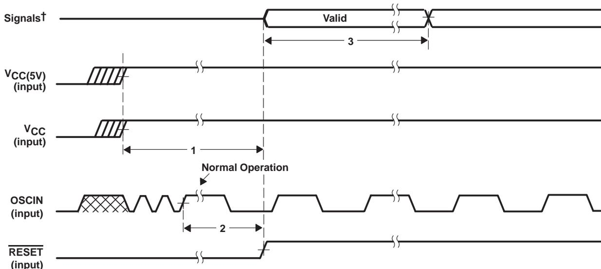
† Outputs are floated during reset. Inputs and I/O's that are not connected to a known logic state at all times, including reset, should have a pullup or pulldown resistor.
