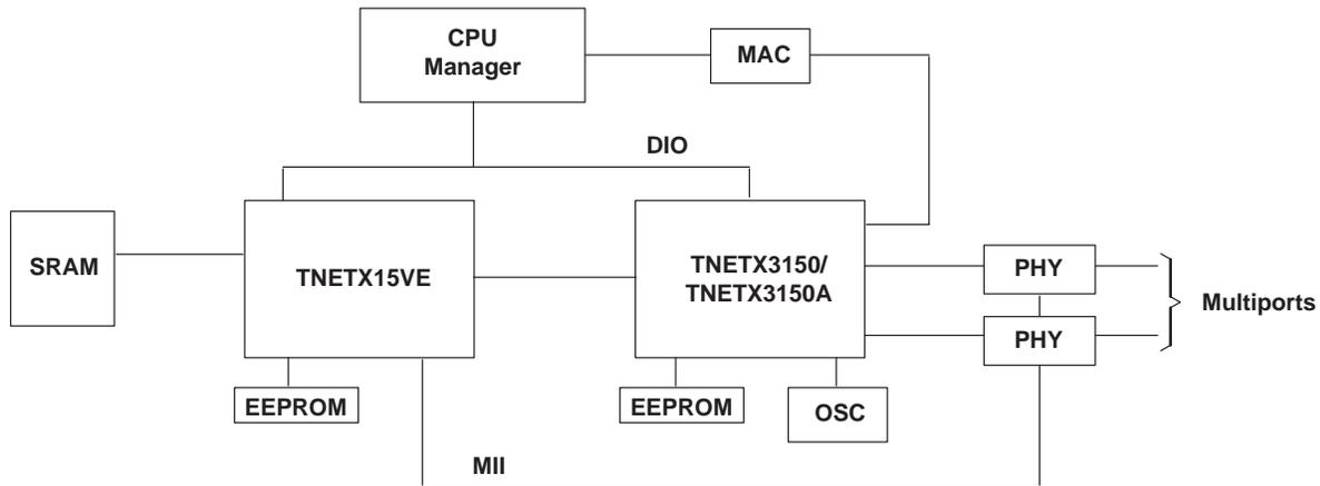
Figure 29. In-Band Managed Multiport Switch
