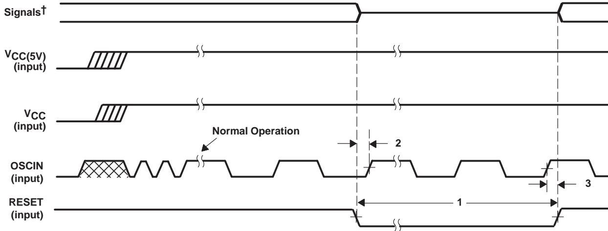
† Outputs are floated during reset. Inputs and I/O's that are not connected to a known logic state at all times, including reset, should have a pullup or pulldown resistor.
