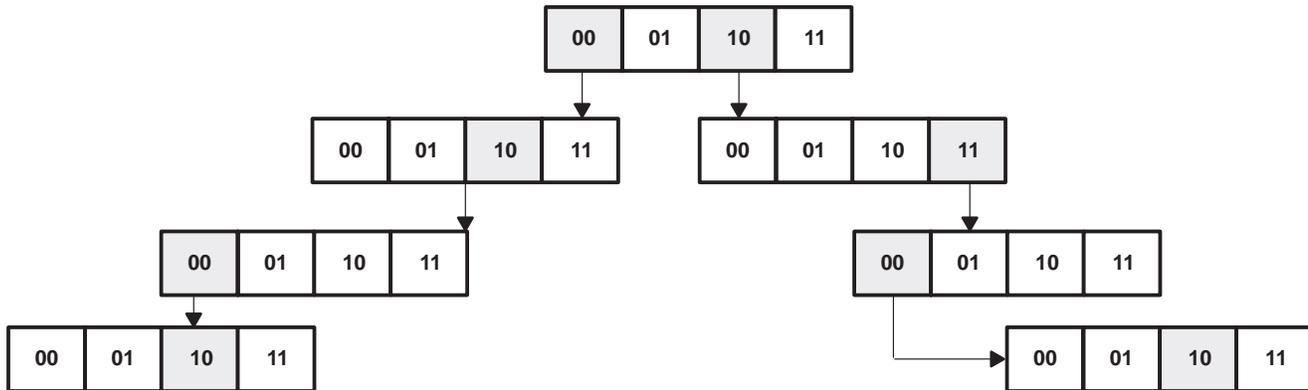
Figure 8. Example of Lookup-Number Algorithm (Adding 0x22)
