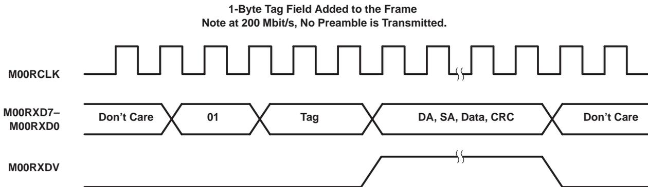
Figure 3. Field Format for Uplink-Port Receive (RX) Frames
