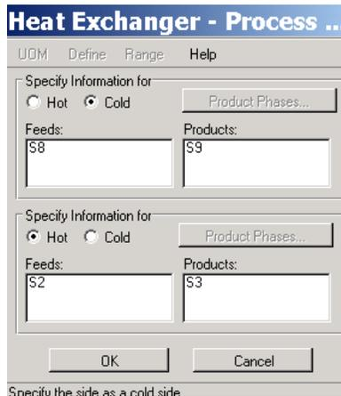
Click on the *OK* button to go back to **PRO/II-Heat Exchanger** window. Click on the *Specification...* button and click on the red box. Choose *Hot Product Temperature* which is the process stream going out of the heat exchanger and type in 90°F for the value.
