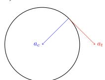
The hawk is now starting to accelerate along the horizontal with a tangential acceleration  $a_t = 1.00 m/s^2$ .
