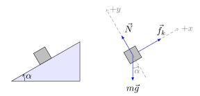
We can use  $x=\frac{1}{2}at^2+v_0t+x_0$  to find the acceleration of the object as it slides down. with  $v_0=$  and  $x_0=0$ . The object slides 1.90 meters in 2 seconds, this should give us:
