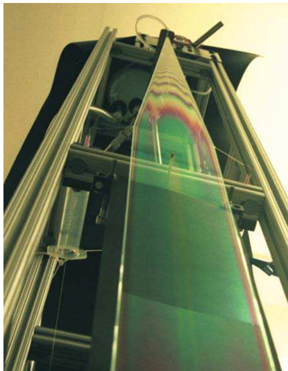
FIGURE 22.6 Huge soap film showing reflection fringes, used to study flow in thin films.
