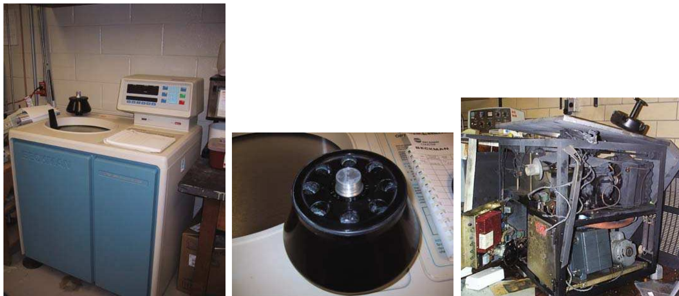
FIGURE 5.27 (upper) Modern ultracentrifuge; (middle) fixed angle rotor; (bottom) centrifuge remains after accident in which a rotor exploded while spinning.
