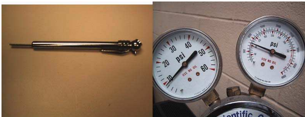
FIGURE 8.23 Tire gauge and high pressure gas gauge used to measure (gauge) pressure.
