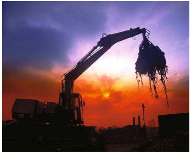
FIGURE 17.21 An electromagnet on a crane used to pick up scrap metal.
