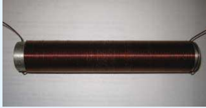
FIGURE 17.23 (left) A solenoid made from winding wire around a metal core; (right) a longitudinal cross-section of the center portion of a solenoid showing the cut windings with current flowing around from the bottom to the top (counterclockwise, as viewed from the left), producing a uniform B field to the left. The rectangular Amperian loop is used to evaluate Ampere's law in order to find the B field inside the solenoid.
