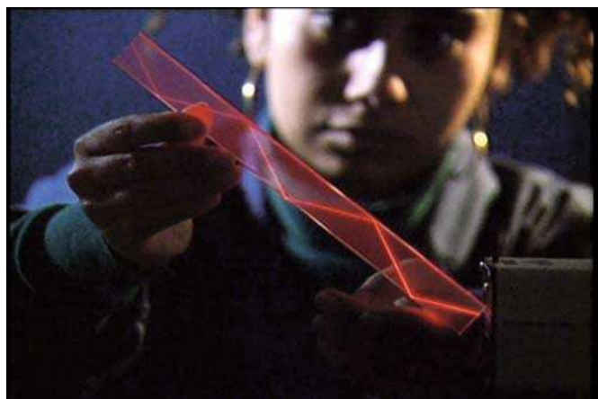
FIGURE 20.20 Total internal reflection in a light pipe.
