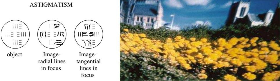
FIGURE 21.10 The four other monochromatic aberrations, other than spherical aberration, with schematics and example photos.
