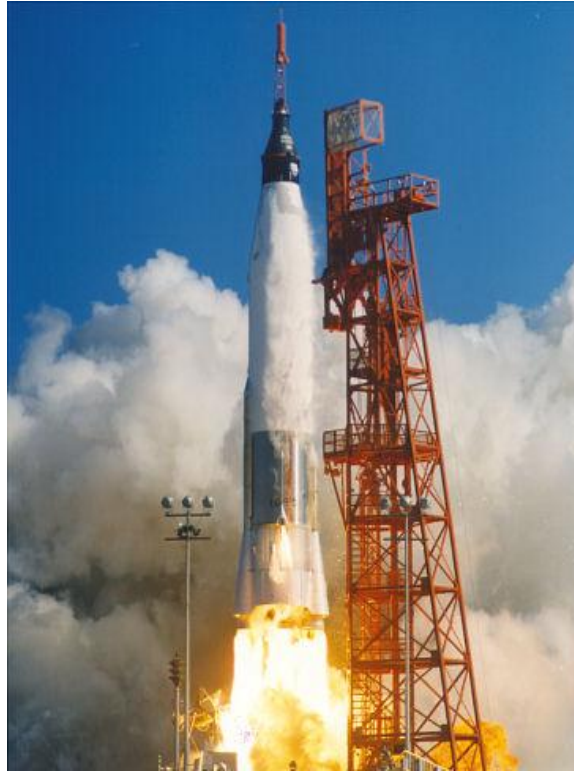
Figure 11.3: The Atlas family of rockets would collapse under their own weight if the fuel tanks were empty.
