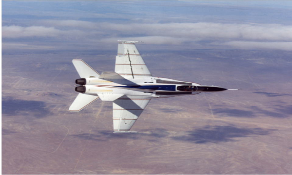
Figure 11.2: The X-53 attempts to use small control surfaces to induce wing-warpage and control the aircraft.
