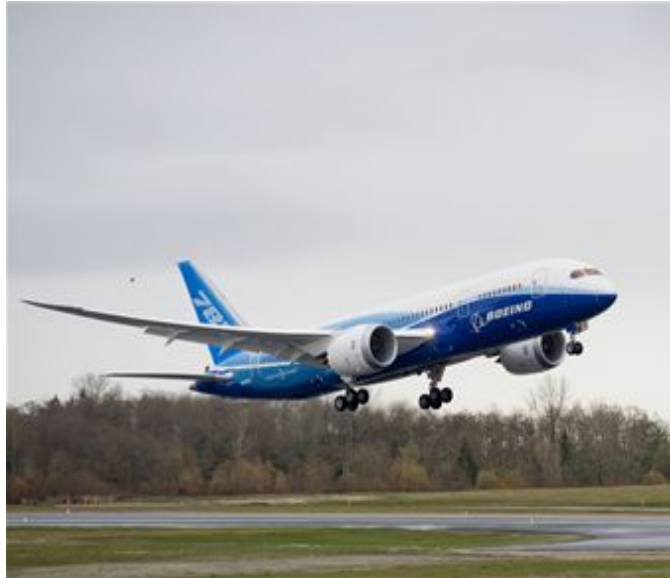
Figure 11.4: The Boeing 787 is the first commercial airliner made mostly of carbon fiber.
