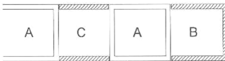
Figure 3.6 Lack of connection between portions of the building or of the aggregate, (Giuffrè 1993). A - Old cell of the aggregate; B - Following addition of a portion of aggregate: later addition; C - Following addition of a portion of aggregate: interclosed cell.
