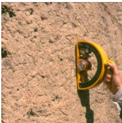
Figure 5.21 Schmidt Hammer to measure Cob hardness, (Source: ZRS).
