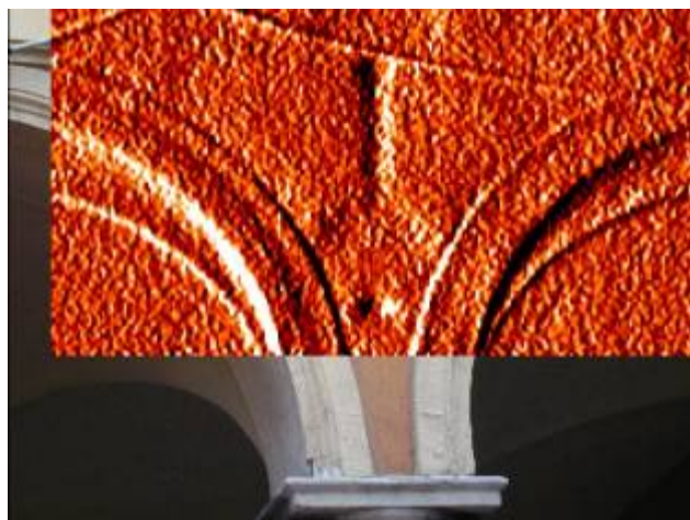
Figure 5.3 Data of Figure 5.2 after the application of a gradient filter to enhance the target, (Binda 2003b)
