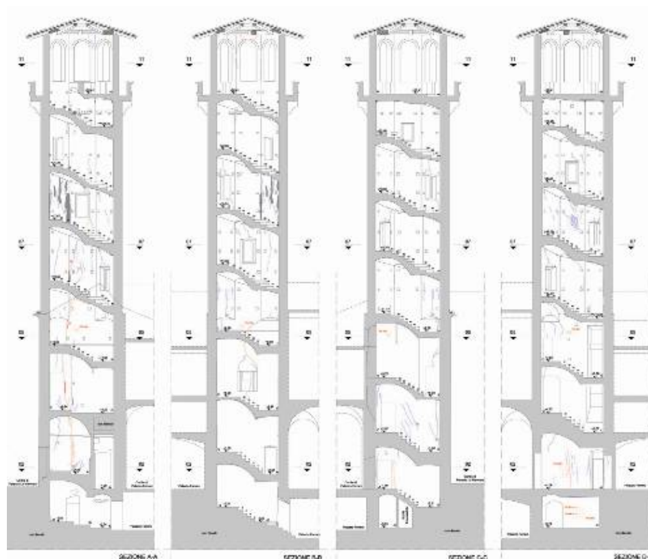
Figure 4.1 Crack pattern survey of the internal prospects of a highly damaged tower in Biella (Italy), (Anzani 2008).
