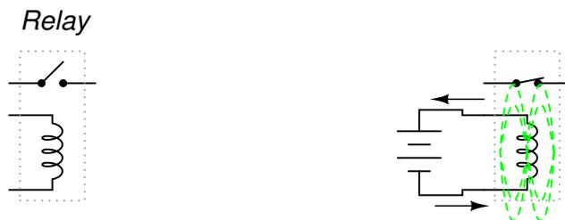
**Applying current through the coil causes the switch to close.**
