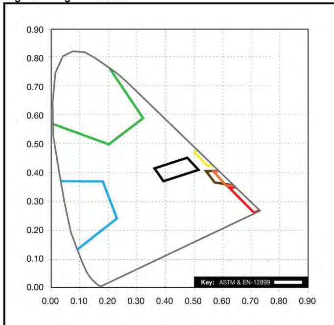
OL-2000 Series Overlay Films **meets** the current applicable daytime and nighttime color requirements for ASTM D4956 and EN 12889.
