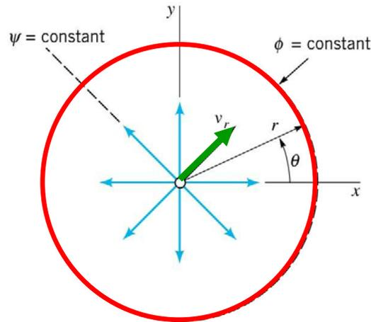
Source/Sink Flow is a purely radial flow.
