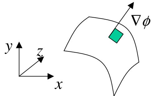
Gradient of a Scalar (i.e., density, temperature,etc)
