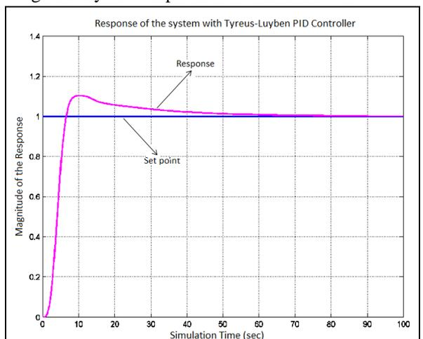
Figure.11 System response with cascaded TL PID
