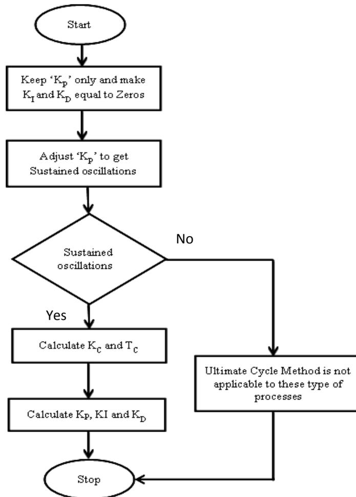
Figure.4 Flow chart for PID tuning procedure
