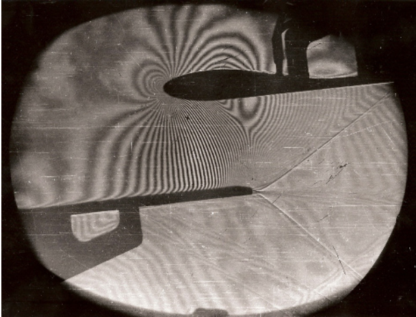
Fig. 11. Interferogram of flow field in the blade cascade representing the section 800 mm from the root at exit isentropic Mach number M_{2is} = 1.503 , inlet angle \beta_1 = 126.8^\circ , and inlet Mach number M_1 = 0.529 .
