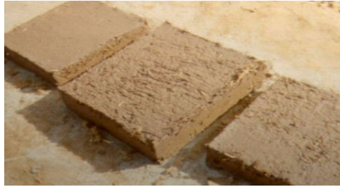
Figure 18. Earth brick samples. Soil, straw, water compressed into a mould then dried.
