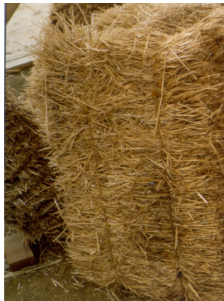
Figure 3. A typical two-string straw-bale.
