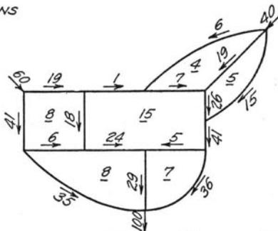
FIG. 3. DISTRIBUTION OF FLOW IN NETWORK—TWO INLETS; METHOD OF BALANCING HEADS
