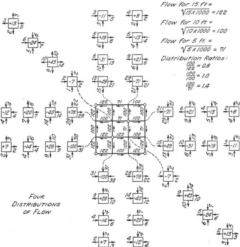
FIG. 7. DISTRIBUTION OF FLOW IN NETWORK—SEVERAL INLETS AND OUTLETS; METHOD OF BALANCING FLOWS
