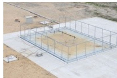
Fire test stand for containment systems of dangerous goods
