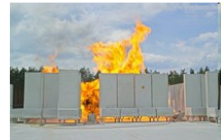
Fire test stand B, heat input test on a 5000-l container
