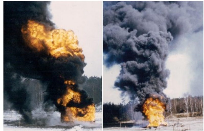
Large scale fire tests with 5 tons TBPB (left) and 5 tons TBPEH
