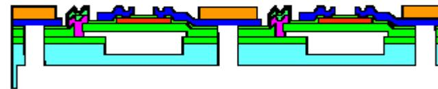
10. Spin, pattern and cure polyimide on the backside. Electroless plate nickel/gold on backside pads.
