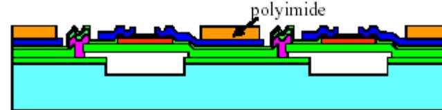
8. Pattern backside; RIE etches nitride; DRIE etches Si to 70 μm thick.
