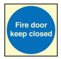
Fire doors are doors that are designed to restrict the spread of fire and the products of combustion within a predicted time period and will normally feature a self closing device. All fire doors are marked as a fire door and should be kept closed at all times. The use of wedges and other items as hold open devices is not permitted within any of the University's premises and must be positively discouraged.
