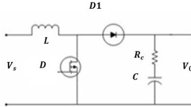
Figure 3: Schematic Configuration of a DC-DC Boost Converter
