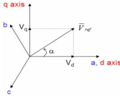
Figure 6: Voltage Space Vector and its Components in (d, q)
