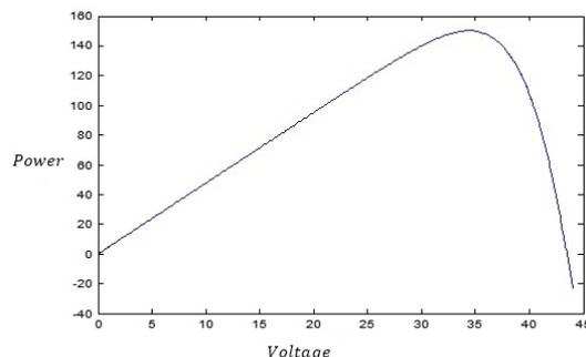
Figure 9: Voltage Power Waveform of PV
