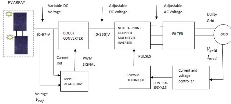
Figure 1: Grid-Connected PV Energy Conversion System and the Associated Closed Loop Control Structure
