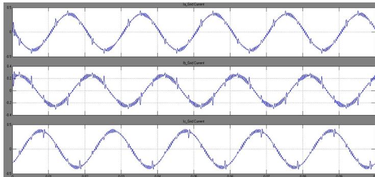
Figure 13: Grid Current Waveform of Current Controller
