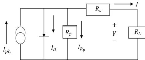
Figure 2: Simplified-Equivalent Circuit of Photovoltaic Cell
