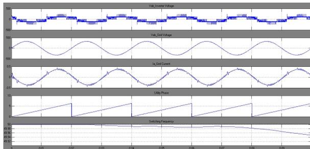
Figure 11: Inverter Voltage, Utility Voltage, Grid Current, Utility Phase Angle and Switching Frequency
