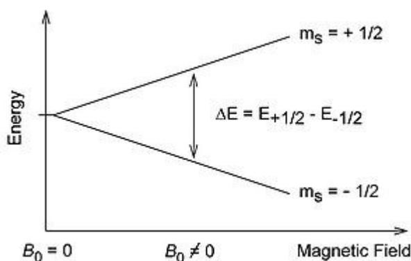
An unpaired electron can move between the two energy levels by either absorbing or emitting a [photon](#) of energy  $h\nu$  such that the resonance condition,  $h\nu = \Delta E$ , is obeyed. This leads to the fundamental equation of EPR spectroscopy:  $h\nu = g_e \mu_B B_0$ .
