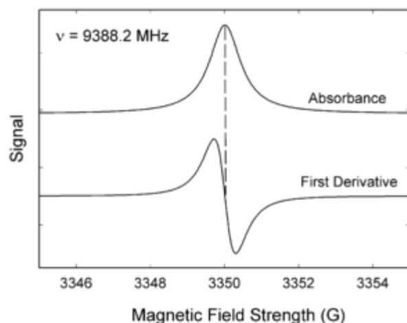
For the microwave frequency of 9388.2 MHz, the predicted resonance position is a magnetic field of about  $B_0 = h\nu/g_e\mu_B = 0.3350 \text{ tesla} = 3350 \text{ gauss}$ .
