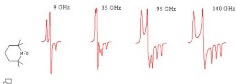
EPR spectra of TEMPO, a nitroxide radical, as a function of frequency. Note the improvement in resolution from left to right. [\[8\]](#)
