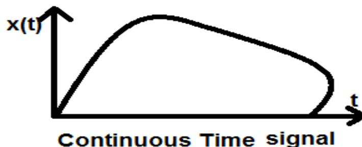
The signal shown above is an example of continuous time signal because we can get value of signal at each instant of time.
