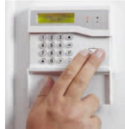
Explain to the customer about the panic alarm. By pressing the two buttons indicated will initiate the internal and external sounders.
