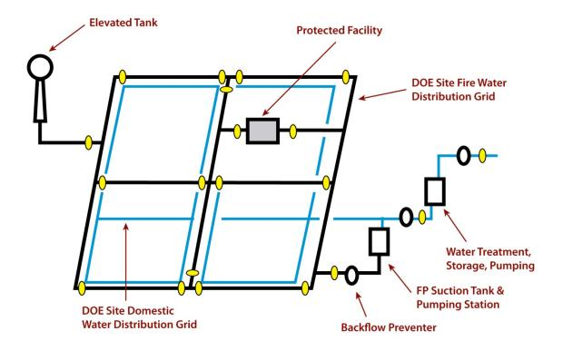
Similar to Arrangement 2, this arrangement should not be utilized for SC applications, but is used for general purpose fire protection and may be used for SS applications, if requirements for reliability, QA, and safe operation are met. The reason the system is not to be used in SC applications is that, even though the system is under DOE control, it is not under the facility's control. Thus having an additional backup system that is under the facility's control is prudent.
