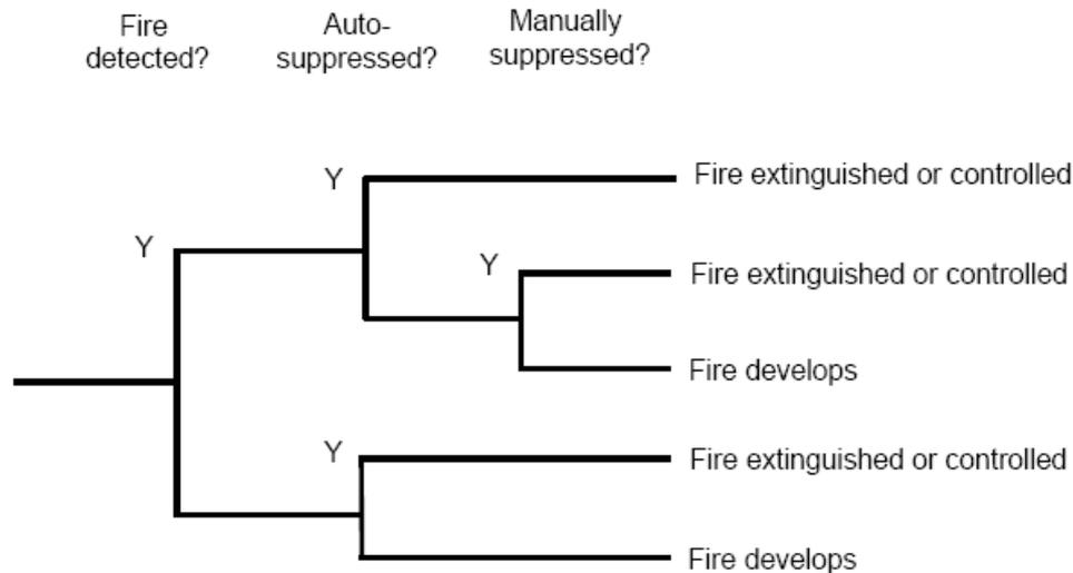
**Figure 1. Fire development event tree (extracted from Houlding and Rew 2003)**
