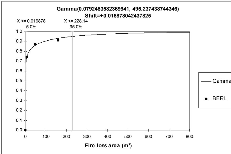
Figure 15. Cumulative distribution function of the fire loss area for an unprotected building
