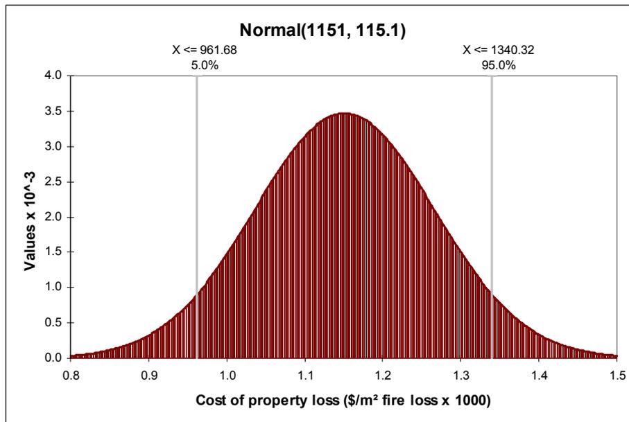
**Figure 32. Probability density function for the cost of direct property losses**
