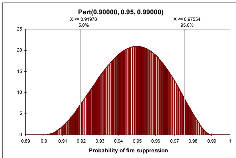
Figure 19. Probability density function for fire sprinkler success
