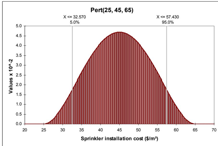
Figure 29. Probability density function for sprinkler installation cost
