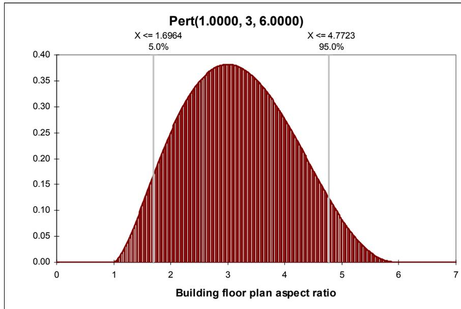
**Figure 26. Probability density function for building plan aspect ratio**
