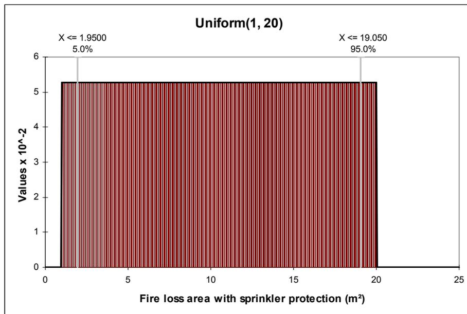
Figure 16. Probability density function for the fire loss area with sprinklers
