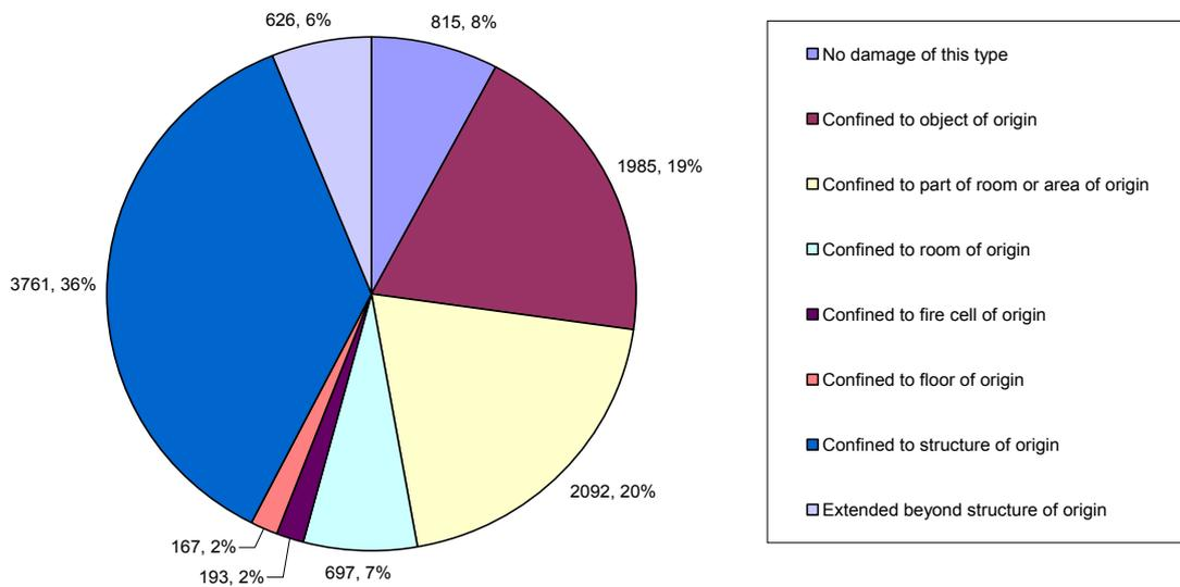
**Figure 12. Structure fires in industrial buildings by extent of flame damage 1986–2005 (Challands 2005)**
