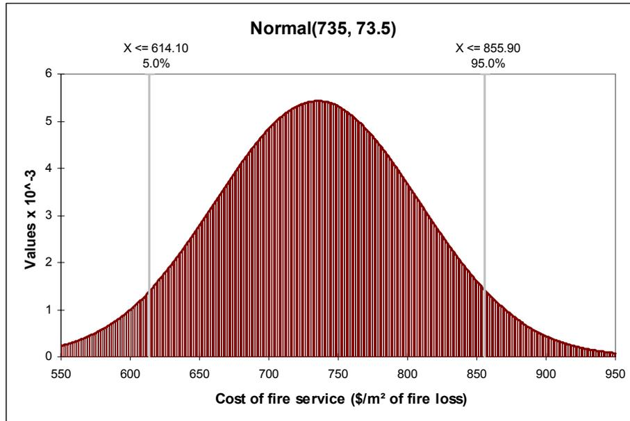
**Figure 33. Probability density function for the cost of the fire service**
