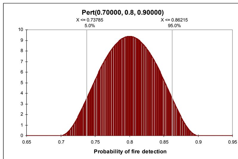
Figure 21. Probability density function for fire detection success
