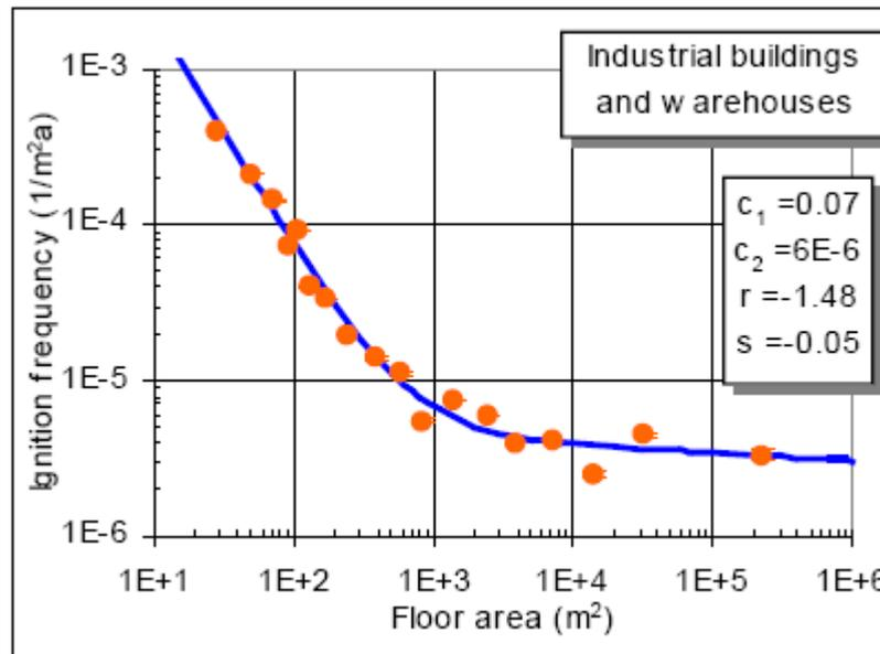
Figure 2. Ignition frequency observations (dots) in industrial buildings and warehouses 1996–1999 Finland and a generalised Barrios model fitted to the data (solid line). Extracted from Tillander and Keski-Rahkonen (2003)
