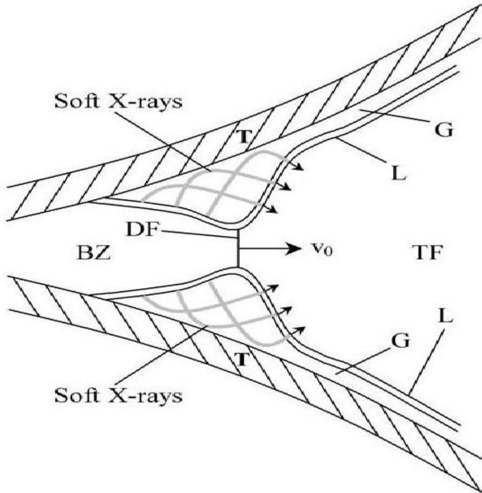
**Fig.5.** Autocatalytic thermonuclear detonation using a soft X-ray precursor from the burn zone BZ to precompress the thermonuclear fuel TF ahead of the detonation front DF. The soft x-rays travel through the gap G between the tamp T and the linear L.
