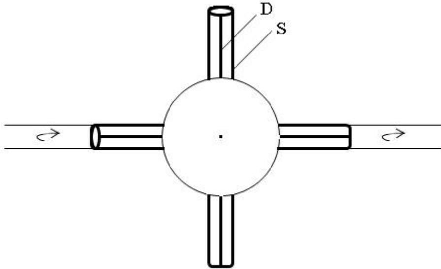
**Fig. 3.** Propagating burn into DT or D placed inside small magnetized superconducting solenoids S, compressed by imploding convergent shock wave.
