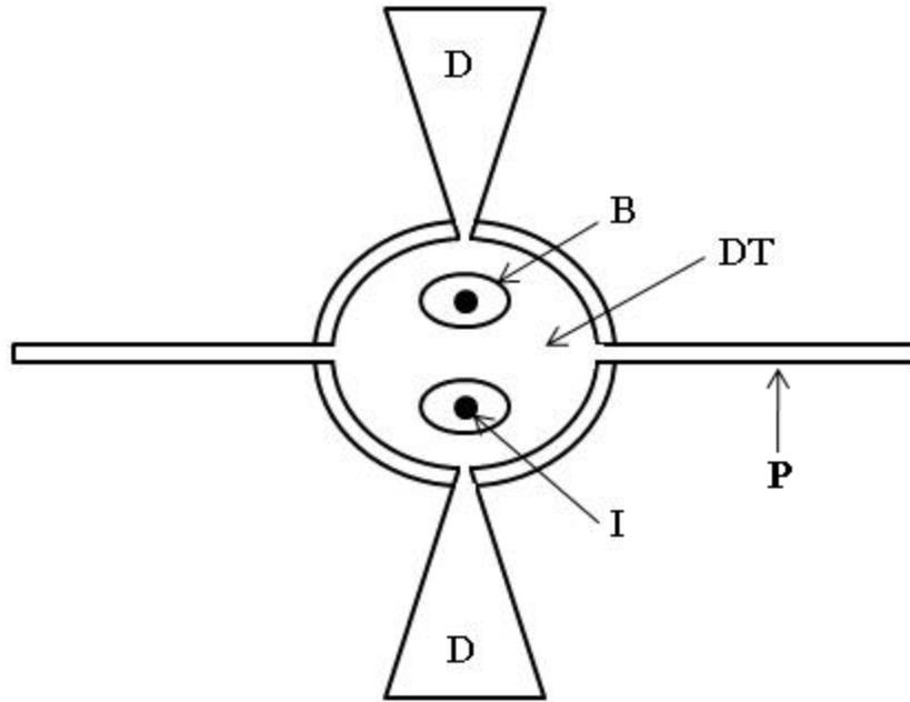
**Fig.2.** Formation of field reversed configuration of magnetized DT target in the center of convergent shock wave. B and I toroidal magnetic field current; P imploded pipe, D solid deuterium.
