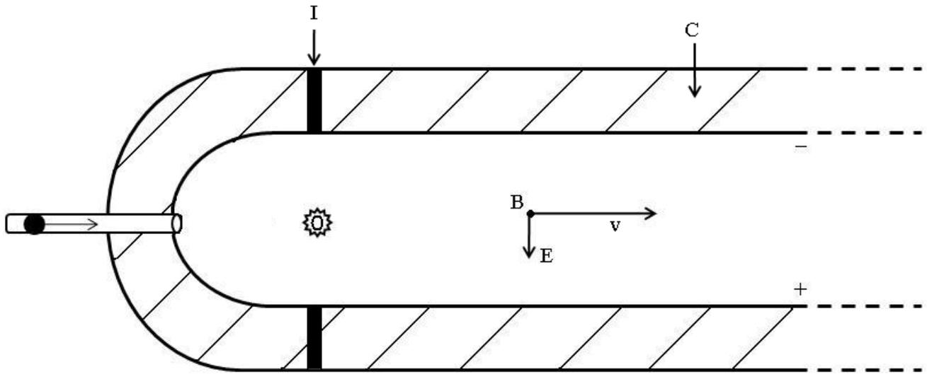
**Fig.6.** Faraday generator for chemical-nuclear energy conversion into electric energy : F hybrid chemical-fusion mini-bomb, B magnetic field directed perpendicular to plane of drawing and produced by electromagnets,  $v$  velocity of plasma fire ball which induces electric field  $\mathbf{E} = (\mathbf{v} / c) \times \mathbf{B}$ , C wall confining plasma flow, I insulator.
