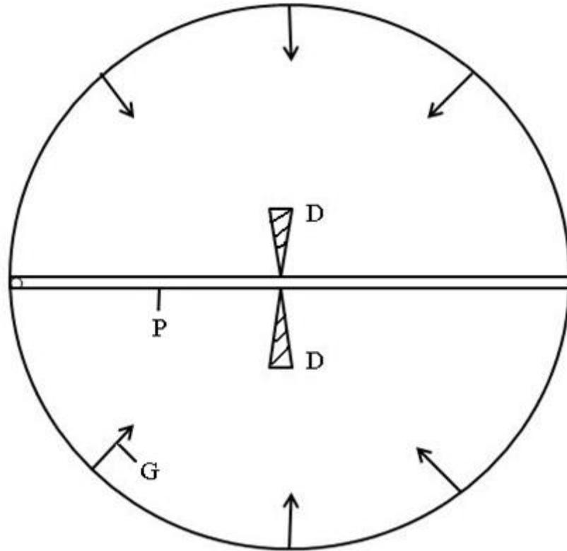
**Fig. 1.** Convergent Gudeley shock wave G onto magnetized fusion target in hollow pipe P with additional deuterium D for propagating burn into a region with an increasing diameter (horn) for a growing thermonuclear detonation wave.
