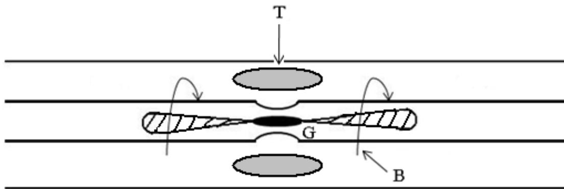
**Fig.4.** Magnetized target T in coaxial conductor, with propagating burn of high gain target G inside inner conductor ignited by magnetized target ; B magnetic field.
