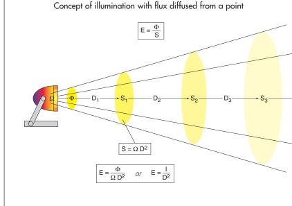
Fig. n. 3 Direct illumination decreases with the square of the distance
