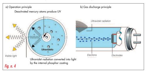
In preheated cathode lamps, the electrodes consist of a tungsten filament and are heated by the current.
