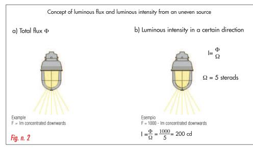
The concept of luminous intensity forms the basis of lighting technology calculation which is based on physically defined elements, known as point by point calculus. It is therefore important to elaborate on this concept by extending it to directional sources.
