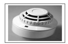
ii) Photoelectric Detector – This type of detector employs the light scattering principle of smoke for detection. A light source (pulsed IR LED) and a light sensor (Photo diode) are arranged in a chamber in such a way that major portion of the light does not fall on the sensor. When smoke particles enter the light path inside the chamber, the light is scattered and this scattered light falls on the sensor which converts it into a signal for further action.
