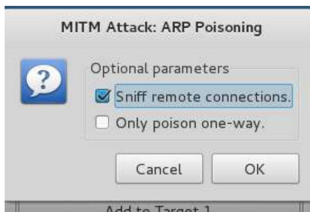
**Step 11:** Click "start" and select "start sniffing". This will start ARP poisoning in the network which means we have enabled our network card in "promiscuous mode" and now the local traffic can be sniffed.
