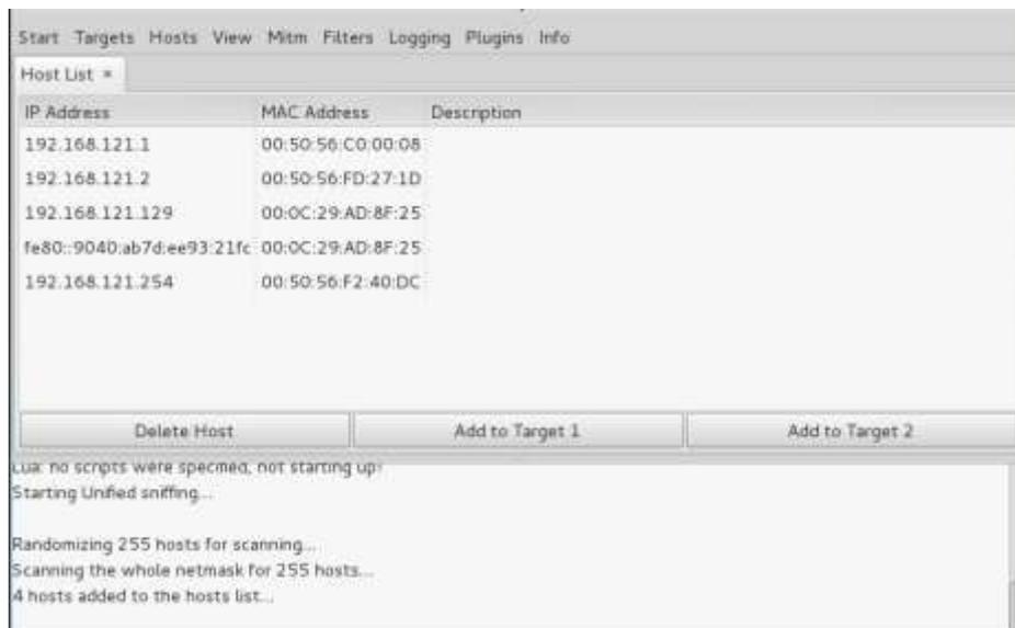
**Step 8:** Now we have to choose the targets. In MITM, our target is the host machine, and the route will be the router address to forward the traffic. In an MITM attack, the attacker intercepts the network and sniffs the packets. So, we will add the victim as "target 1" and the router address as "target 2."
