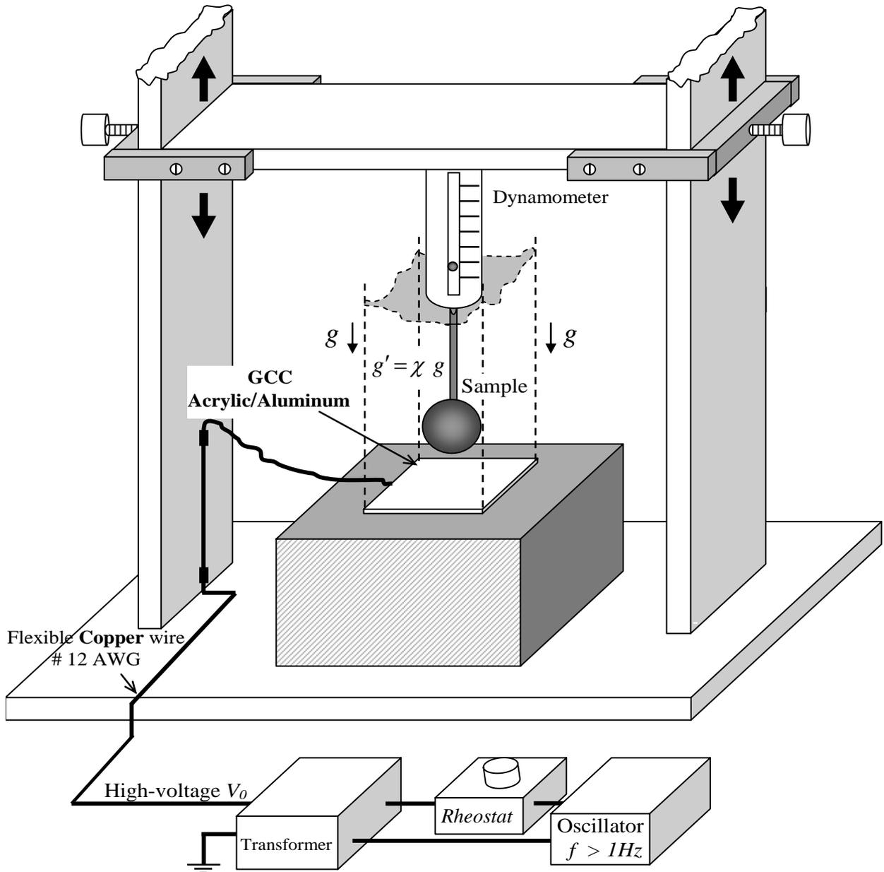
Figure A9 – *Experimental Set-up using a GCC subjected to high-voltage  $V_0$  with frequency  $f > 1\text{Hz}$ . Note that in this case, the pan balance is not necessary because the substance of the Gravitational Shielding is an air layer with thickness  $d$  above the acrylic sheet. This is therefore, more a type of Gravity Control Cell (GCC) with external gravitational shielding.*
