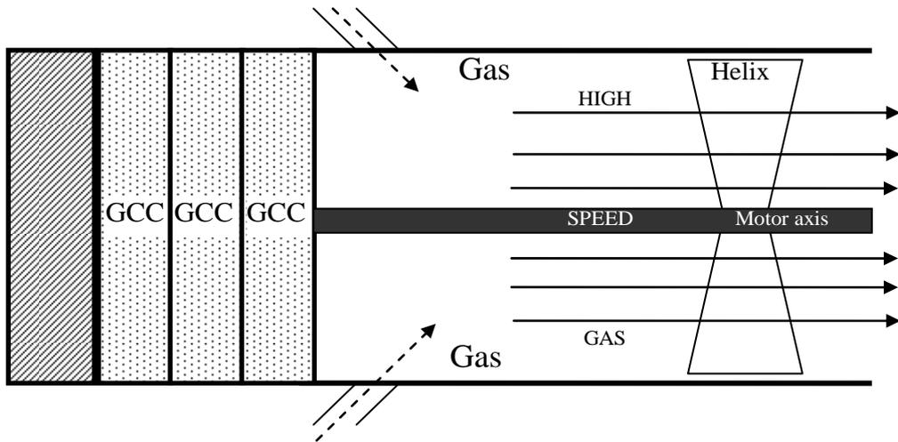
Fig. 12 - The Gravitational Turbo Motor – The gravitationally accelerated gas, by means of the GCCs, propels the helix which moves the motor axis.
