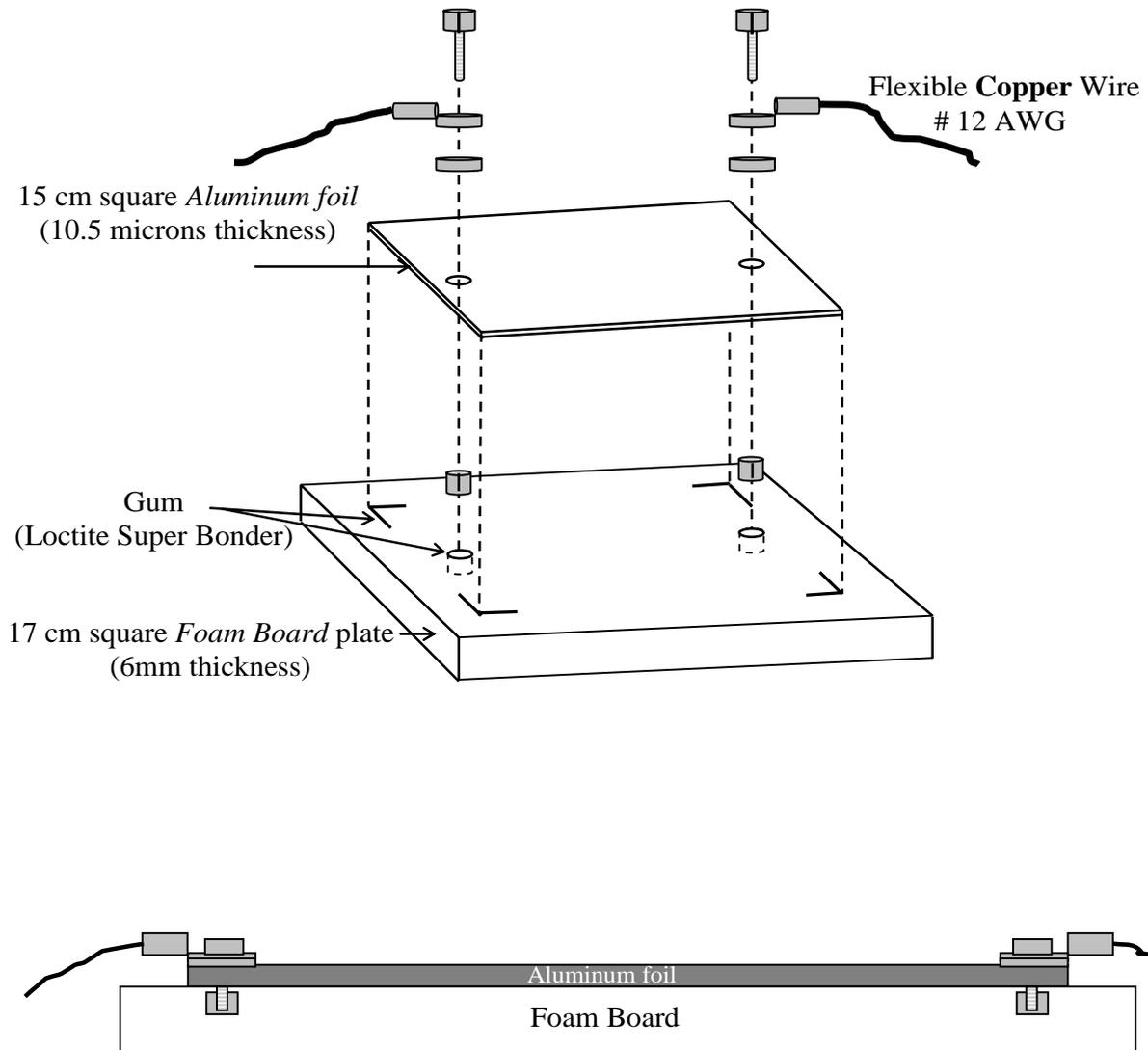
Figure A3 – The Simplest *Gravity Control Cell* (GCC).
