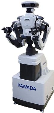
**“ITS ‘HEAD’ IS EQUIPPED WITH STEREO VISION JUST LIKE A HUMAN. THIS MEANS THAT NEXTAGE CAN ATTAIN 3D COORDINATES WITH HIGH PRECISION.”**
