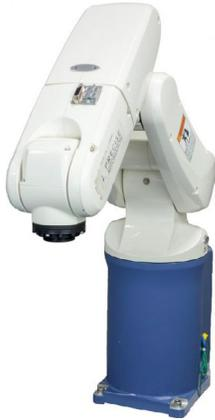
*“[...] ALL CONTROL ELECTRONICS AND POWER SUPPLIES ARE BUILT INTO THE ROBOT'S BASE CREATING AN EXTREMELY COMPACT STRUCTURE THAT ELIMINATES EXTRA CONTROLLER CABINETS, EXTERNAL HARNESSING AND COMPLICATED INSTALLATIONS AND INTEGRATIONS.”*
