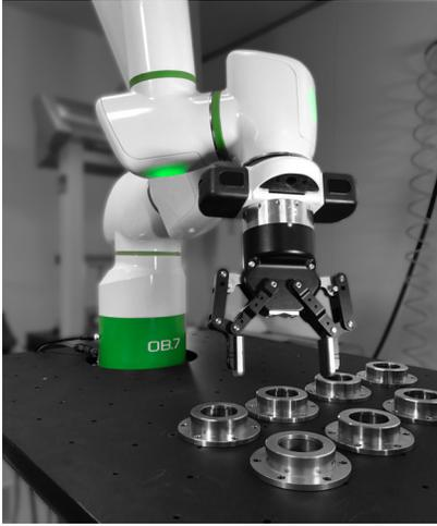
*"MOVES SIMILARLY TO THE HUMAN ARM WITH SEVEN JOINTS, ONE METER REACH, AND THE ABILITY TO LIFT 5KG OR 11LBS. OB7 IS ABLE TO MANEUVER INTO TIGHT SPACES AND CAN EASILY ADAPT TO YOUR EXISTING MANUFACTURING ENVIRONMENT."*
