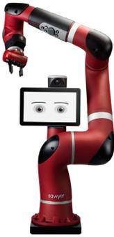
**“SAWYER IS MORE PRECISE THAN BAXTER AND ALSO HAS BETTER REPEATABILITY, WHICH IS PARTLY DUE TO THE NEW ZERO BACKLASH GEAR BOXES AND HARMONIC DRIVE MOTORS BEING USED.”**
