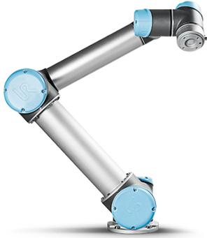
**THE LIGHTWEIGHT, FLEXIBLE AND COLLABORATIVE INDUSTRIAL ROBOT - UR5 - FROM UNIVERSAL ROBOTS LETS YOU AUTOMATE REPETITIVE AND DANGEROUS TASKS WITH PAYLOADS OF UP TO 5 KG.”**
