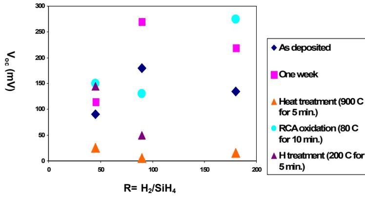
Fig. 15. Open-circuit voltage with hydrogen dilution after various post-deposition treatments.
