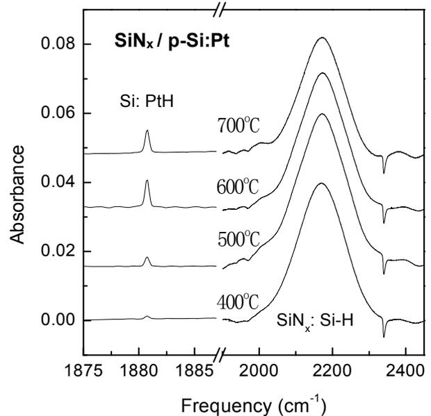
Fig. 3. Creation of Pt-H complexes in bulk Si by annealing of hydrogenated SiN<sub>x</sub> layer; annealing times of 10 min were used.
