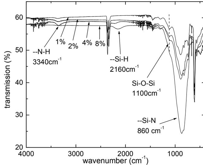
Fig. 1. FTIR transmission spectra of films grown under different SiH<sub>4</sub>/NH<sub>3</sub> flow ratios (indicated in %).
