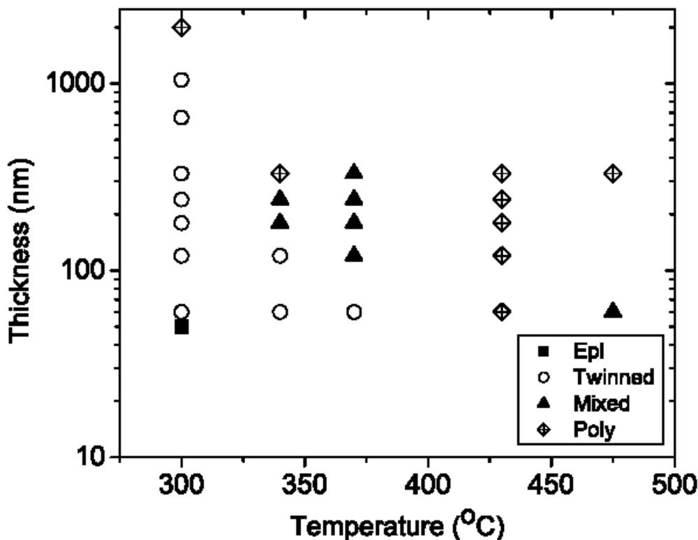
Fig. 6: Phase diagram of HWCVD films grown at 50:1 hydrogen dilution with 4% SiH<sub>4</sub> in He.
