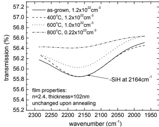
Fig. 2. FTIR spectrum at various annealing temperatures for a film grown with 8%  $\text{SiH}_4$  in  $\text{NH}_3$ ; annealing times of 5 min were used.
