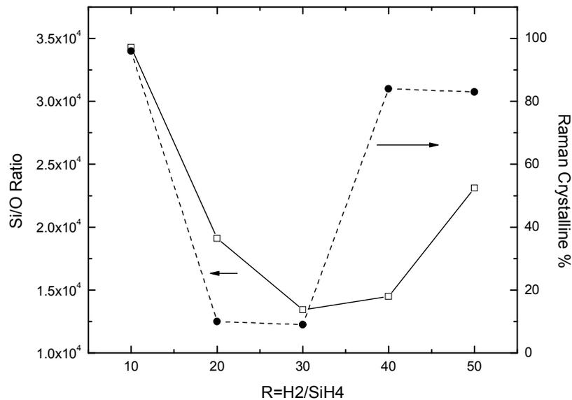
Fig. 11. Silicon to oxygen ratio in the first monolayer of growth as a function of R for pure silane growth using the deposition conditions in Table 4 along with the Raman crystalline %.
