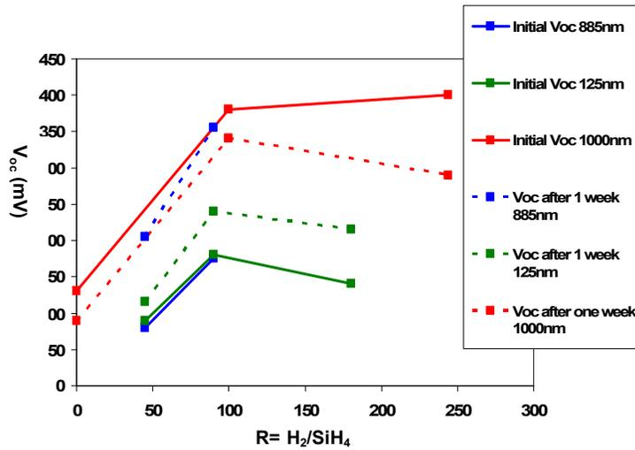
Fig. 14.  $V_{oc}$  with hydrogen dilution immediately after deposition and after one week in ambient air.
