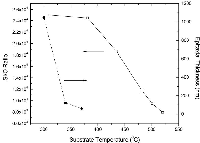
Fig. 10. Silicon to oxygen ratio in the first monolayer of growth as a function of substrate temperature for dilute silane growth at 50:1 hydrogen dilution and epitaxial thickness.
