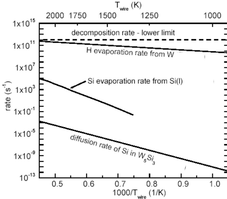
Fig. 5. Rates of interest for wire surface kinetic processes.
