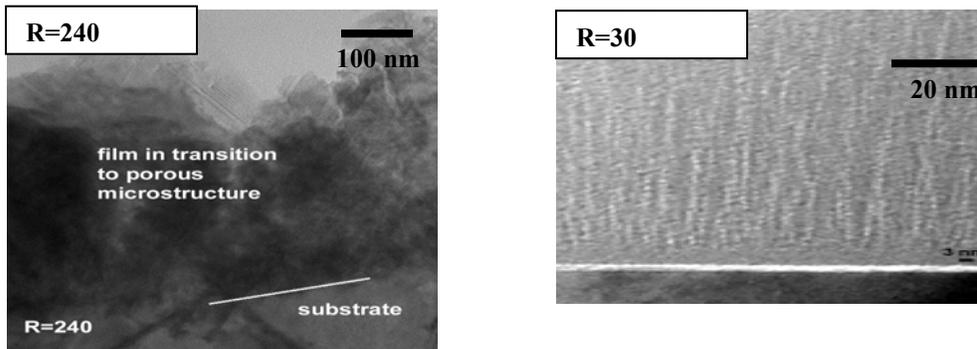
Fig. 13. Cross-sectional TEM of growth morphology at various hydrogen dilutions<sup>26</sup>.
