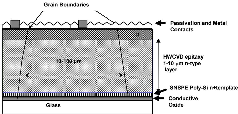
Fig. 12. Schematic of proposed photovoltaic device incorporating epitaxial Si growth on a large-grained polycrystalline template fabricated by SNSPE.
