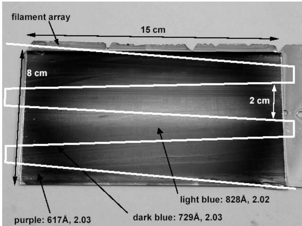
Fig. 4. Photomicrograph of silicon nitride-passivated String Ribbon solar cell; white line depicts position of the wire array during hot wire CVD growth
