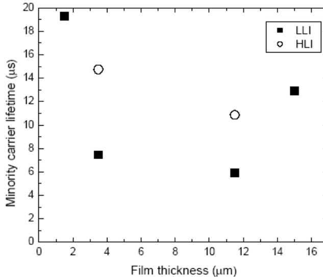
Fig. 9. LLI and HLI minority carrier lifetimes on SNSPE templates.
