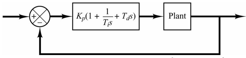
$$\frac{U(s)}{E(s)} = G_{PID}(s) = K_P + K_I \frac{1}{s} + K_D s = K_P \left( 1 + \frac{1}{T_I s} + T_D s \right)$$
