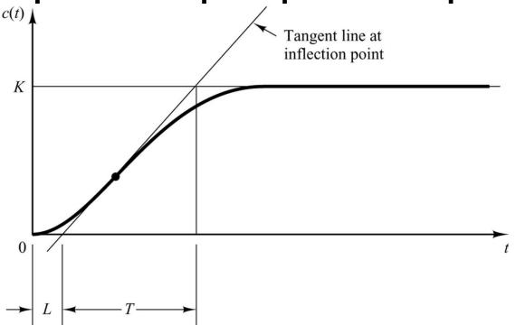
• The S-shaped reaction curve can be characterized by two constants, delay time *L* and time constant *T*, which are determined by drawing a tangent line at the inflection point of the curve and finding the intersections of the tangent line with the time axis and the steady-state level line.
