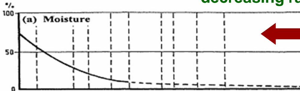
**Moisture content** is determined by heating an **air-dried coal sample** at **105°–110° C (221°–230° F)** under specified conditions until a constant weight is obtained
