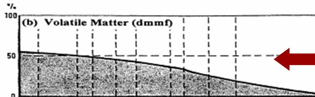
**Volatile matter** is material that is driven off when coal is **heated to 950° C (1,742° F)** in the **absence of air** under specified conditions. It is measured practically by determining the loss of weight
