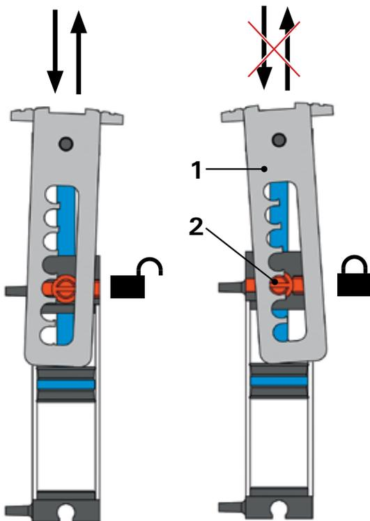
You may use the latch bar (1) to fix the control cylinder at a desired position. This works simply by snapping the latch bar (1) in the strut adapter (2).
