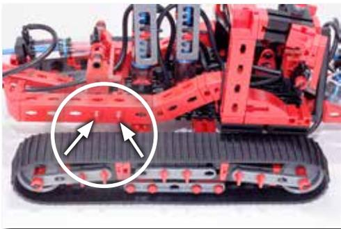
3rd Loosen and remove both the S-bolts on the right.
