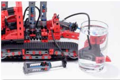
Now you can easily get to all the control cylinders to fill the individual systems with water.
