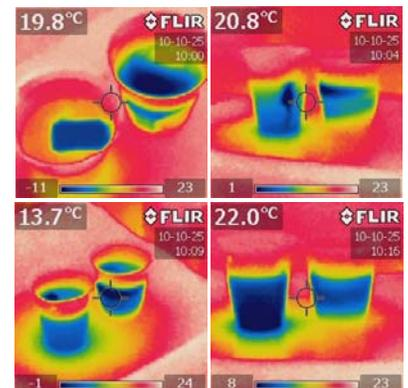
*Figure 14: Seeing the thermohaline stratification. This experiment used just a cup of tap water, a cup of salt water, and some ice cubes. The two cups were placed next to each other on a table for comparison.*
