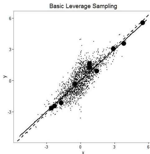
Fig. 3 Example of the Basic Leverage Sampling Method. The data are the same that in Figure 1. The small dots are the original data; the big dots are the sample. The solid line represents the fitted regression line of the full data, and the dashed line represents the fitted regression line of the subsamples.
