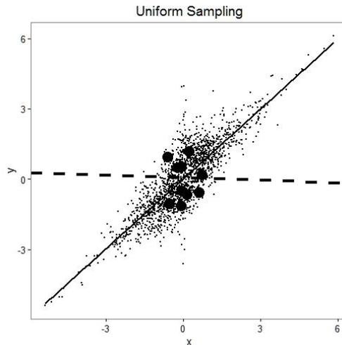
Fig. 1 Example of the failure of the Uniform Sampling Method. For  $i = 1, \dots, 2000$ ,  $y_i = -0.5 + x_i + \varepsilon_i$ , where  $x_i$  is generated from t-distribution with  $df = 6$  and  $\varepsilon_i \sim N(0,1)$ . The small dots are the original data points; big dots are the subsample points. The solid line represents the fitted regression line of the full data, and the dashed line represents the fitted regression line of the subsamples.
