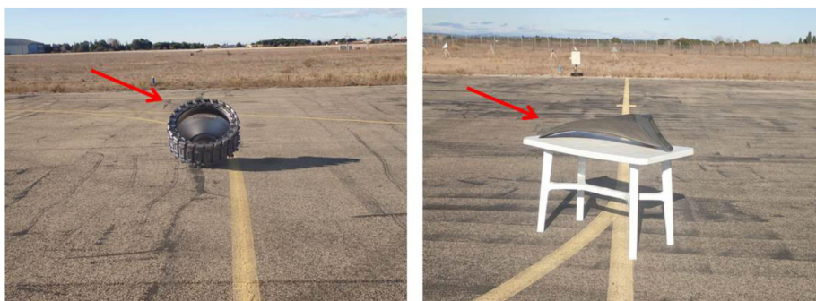
Fig. 41: a fan hub and a fan blade on Nîmes-Garons airport for detection testing
