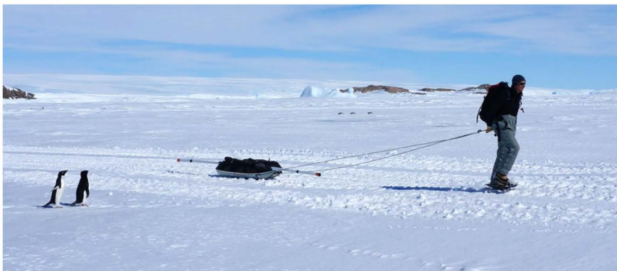
Fig. 35: example of operation of EM31-MK2 in icy conditions
