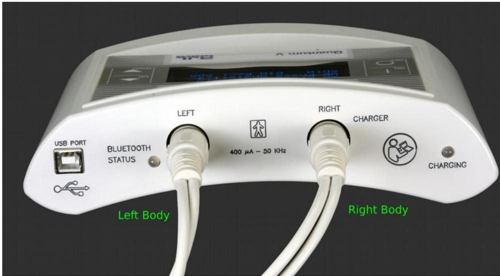
Connect the USB cable to the USB PORT on the back of the Quantum V to a laptop computer with the Segmental BIA application installed
