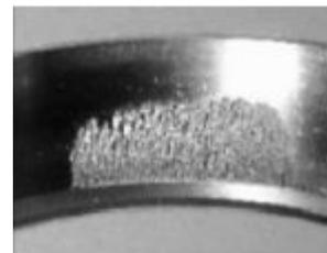
Fig. 4 Outer race defect of bearing 1 of testing 2.
