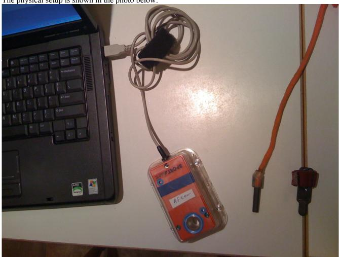
We see here the master control unit on the left, the small coupling stick (needed with the BSF-8 units), and a regular epunch stick (needed to turn the control units on).
