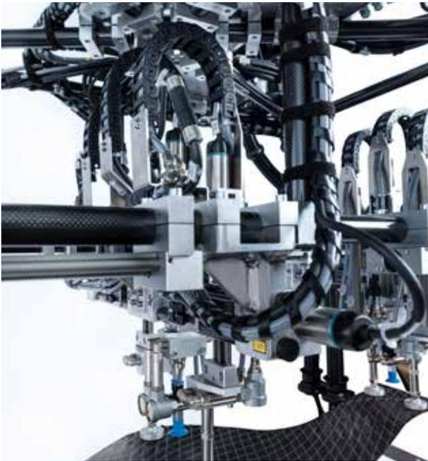
"Differently to e.g. pneumatic systems, the servo technology enables different linear positions to be moved to in a flexible way without any mechanical conversion operations. That was decisive for the process."
