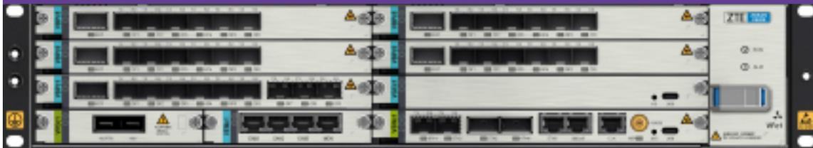
The reference architecture that we have chosen to use is representative of a multi-slot 5G BBU chassis solution where multiple baseband processing cards may be used within a single chassis. The reference architecture refers to the combination of one baseband processing card and one transport/timing card.
