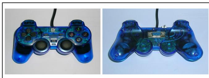
Figure 2. A DualShock-like USB joystick (left) and a hacked joystick showing the nine-pin D-sub-miniature connector mounted underneath the controller and the analog joystick axis switch (right).
