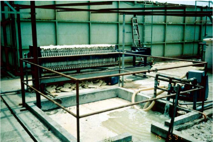
Fig. 6.5.4. Filter press used to dewater zinc sludge. Some of the resulting sludge cake can be seen beneath the press. The zinc has been precipitated out of the wastewater prior to anaerobic and aerobic treatment.
