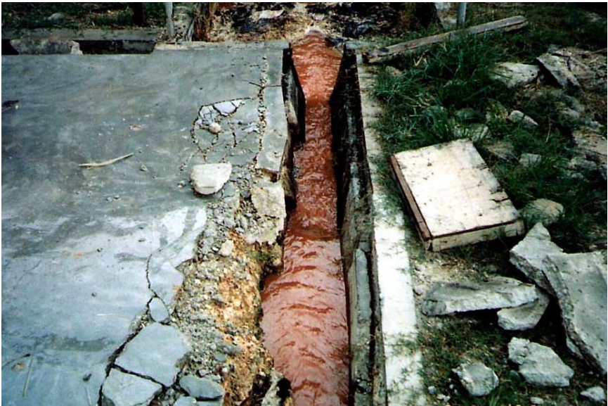
Fig. 9.4.1. A higher than usual amount of blood in the wastewater (red coloration). This was the result of poorer than usual recovery at the slaughterhouse.
