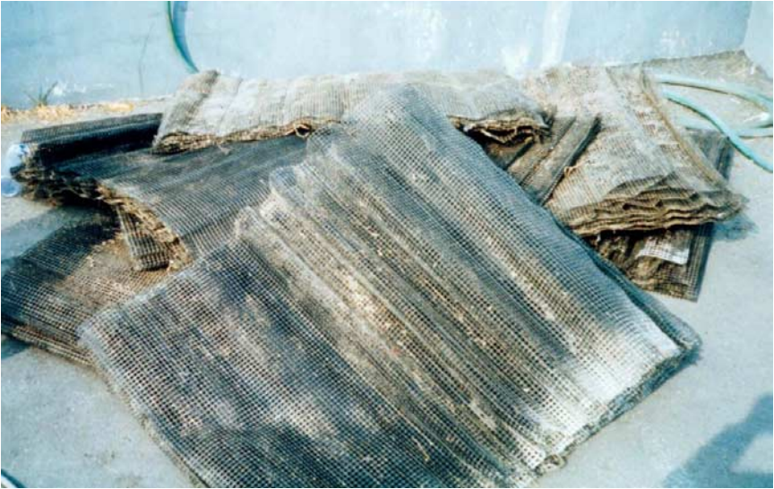
Fig. 5.4.1. Plastic netting-like material which can be assembled into blocks of support medium for biofilm formation.
