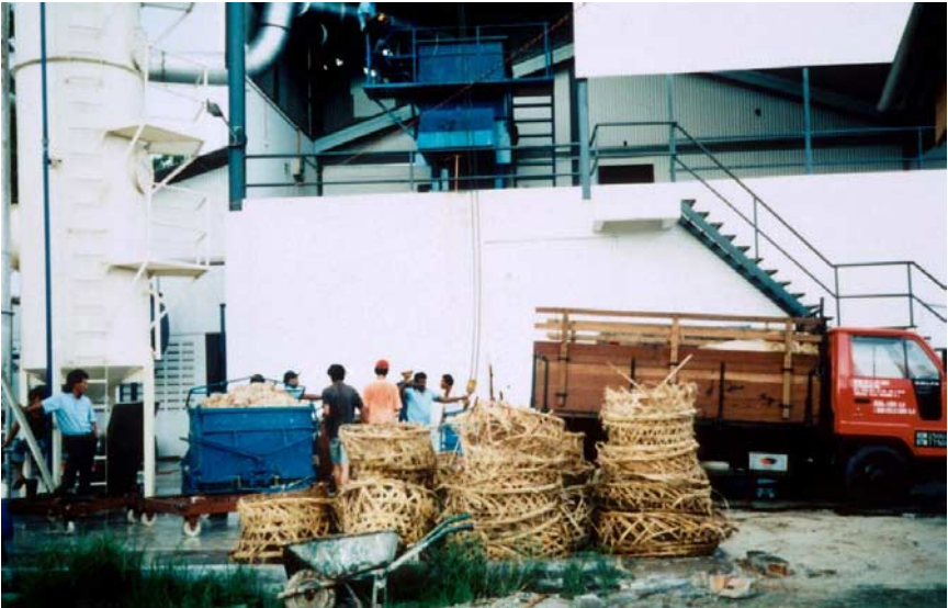
Fig. 9.3.1. Resource recovery from slaughterhouse wastes — feathers. The feathers are collected in the bamboo baskets in the foreground of the picture. Typically the recovered feathers are removed from the slaughterhouse daily.
