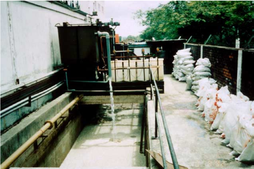
Fig. 4.4.2. Coagulant assisted DAF (top LHS) treating milk canning wastewater. The pretreated wastewater is discharged directly into the bioreactor beneath the DAF for further treatment. The bags on the RHS contain dewatered sludge which was mainly made up of coagulation sludge from the DAF.
