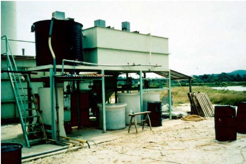
Fig. 4.6.1. A physico-chemical plant for zinc and latex removal. Precipitation (for zinc removal) and coagulation-flocculation (for zinc and latex removal) preceded the DAF (elevated rectangular tank on the RHS). The DAF separated solids generated from the liquid stream. The resulting liquid stream was further treated with bioprocesses.
