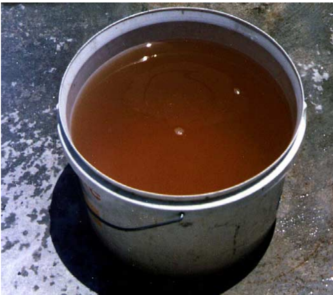
Fig. 8.4.2. Strongly colored treated piggery wastewater. This would have a low BOD but a COD which exceeded the discharge limit.
