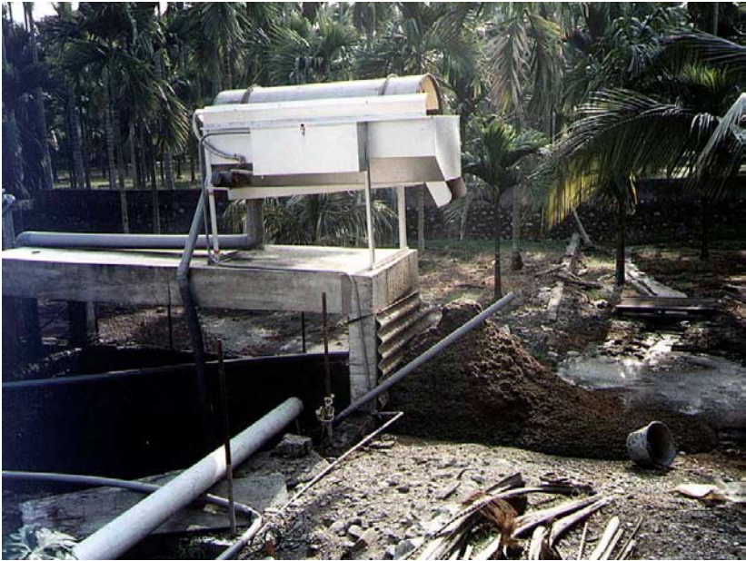
Fig. 4.4.5. Drum-type mechanical fine screen at a pig farm. The screenings below the mechanical screen are not biologically stable and have to be further treated. This may involve composting or liming.
