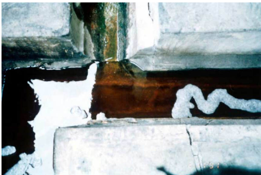
Fig. 10.4.1. Although treated PORE has good clarity, it is strongly colored (brown). The BOD and SS of such a treated wastewater can be very low and can easily meet discharge limits of 20:20. The difficulty lies with the residual COD.
