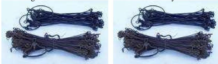
Chains are made up of links which measure 200mm from centre to centre of each middle connecting ring and surveying brass handles are fitted at each end. Tally markers made of plastic or brass are attached at every whole metre position or at each tenth link. To avoid confusion in reading, chains are marked similarly from both end (E.g. Tally for 2m and 18m is the same) so that measurements may be commenced with either end of the chain
