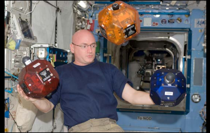
SPHERES robot project uses CO 2 bursts for propulsion
